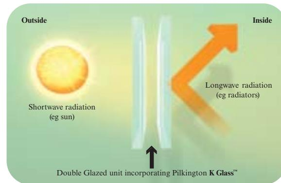
Windows incorporating Pilkington **K Glass™** allow heat from the sun through and reflect heat from fires and radiators back inside, making it easier to keep houses warm.
